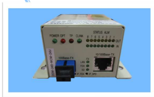
IP optical transmission equipment
